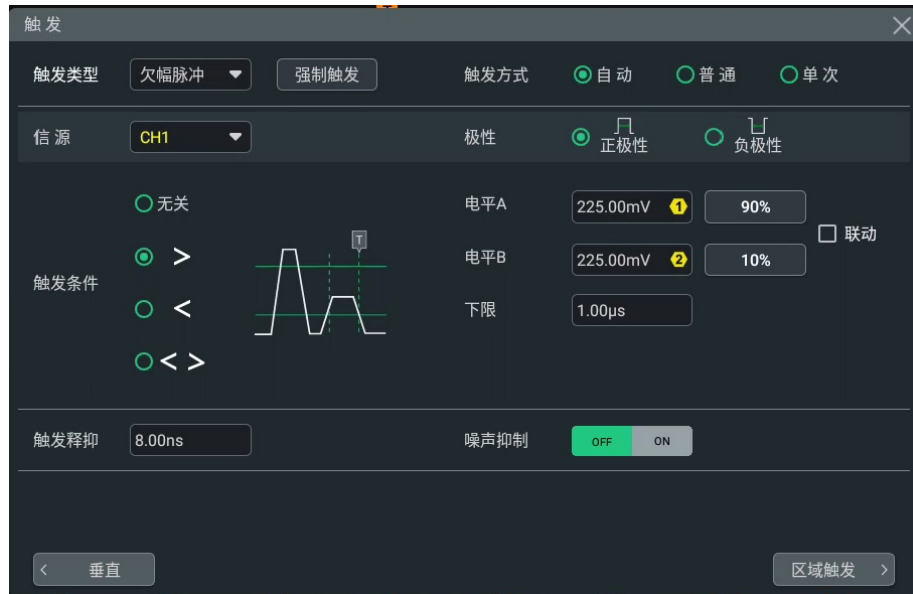
图 8.18 欠幅脉冲触发配置菜单
